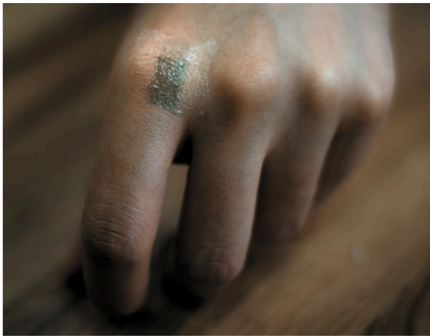
Unobtrusive 'elastronic' transistors can behave like skin and stretch without tearing.
